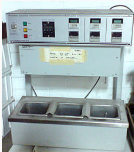
Figure 1b: An older model three-temperature thermal cycler for PCR
