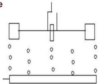
> The sparger ring must be located below the agitator and will have approximately the same diameter as the impeller.
