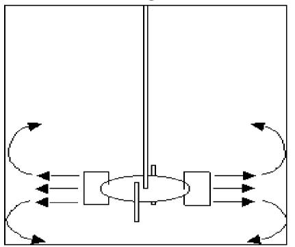
With radial flow impellers, the liquid is pushed towards the wall of the tank; that is, along the radius of the reactor
