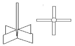
The liquid flow from the blades is directed towards the walls of the reactor; i.e. along the radius of the tank.
