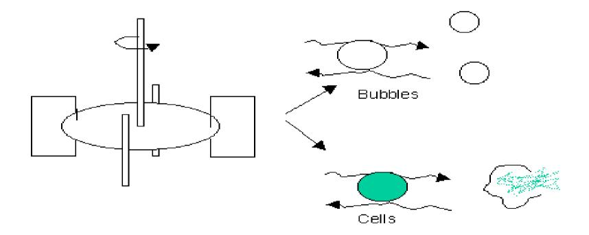
The high shear is effective at breaking up bubbles. For this reason, radial flow impellers are used for the culture of aerobic bacteria.
