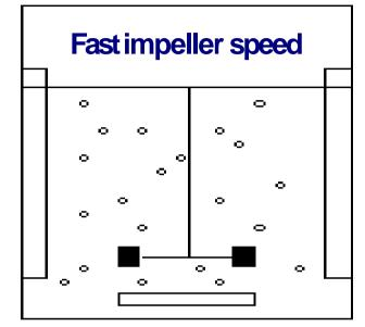
Smaller bubbles will be generated and these bubbles will move with throughout the reactor increasing the gas hold up and bubble residence time
