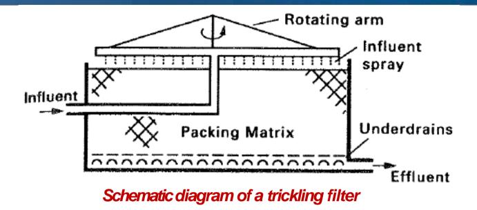
Because trickling filters do not have both a high specific area and a high voidage, they are less suitable for the treatment of large volumes of strong industrial effluents.
