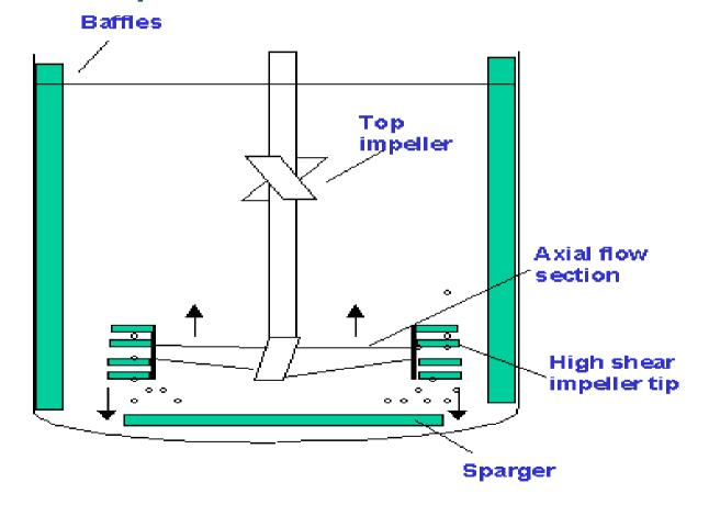
The agitation system has two impellers. The bottom impeller has a large axial flow section. The tips of the impeller contain finger like extensions which create a turbulent wake for breaking bubbles.
