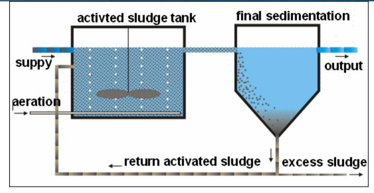
Aeration and Mixing mechanical devices consist of equipment that allow a deeper contact between air and mixed liquor into the tank. Basically, mechanical aerators can be classified into two types: *Mechanical aerators with vertical axis* & *Mechanical aerators with horizontal axis*.
