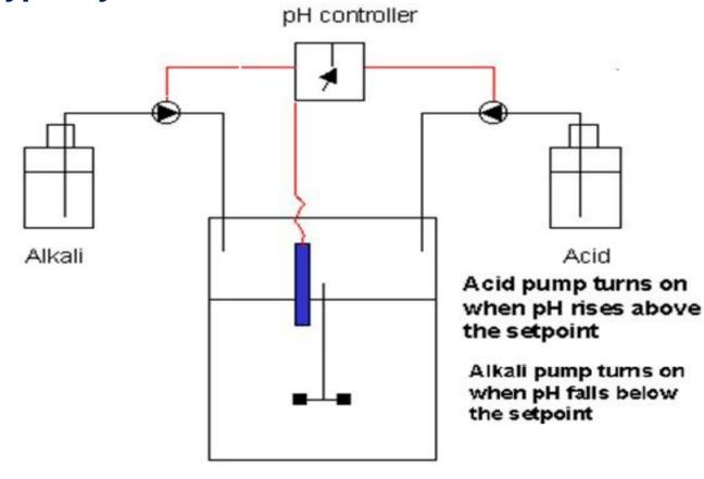
The pH control system (and indeed all other fermenter control systems) are designed to have a dead-band. A dead-band is used to prevent excessive alkali and acid addition. The pH control dead-band is shown in following diagram:
