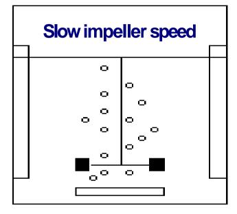
The bubbles will not be sheared into smaller bubbles and will tend to rise directly towards the surface
