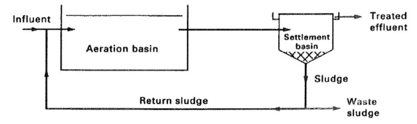
Simplified cross-section of an activated sludge process.
