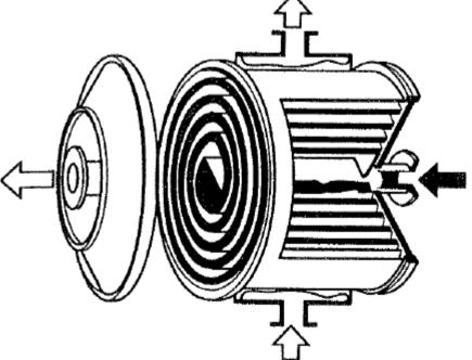
To achieve sterilization temperatures steam is passed through one spiral and medium through the other in countercurrent streams. Spiral heat exchangers are also used to cool the medium after passing through the holding coil. Incoming unsterile medium is used as the cooling agent in the first cooler so that the incoming medium is partially heated before it reaches the sterilizer and, thus, heat is conserved. The major advantages of the spiral heat exchanger are:
