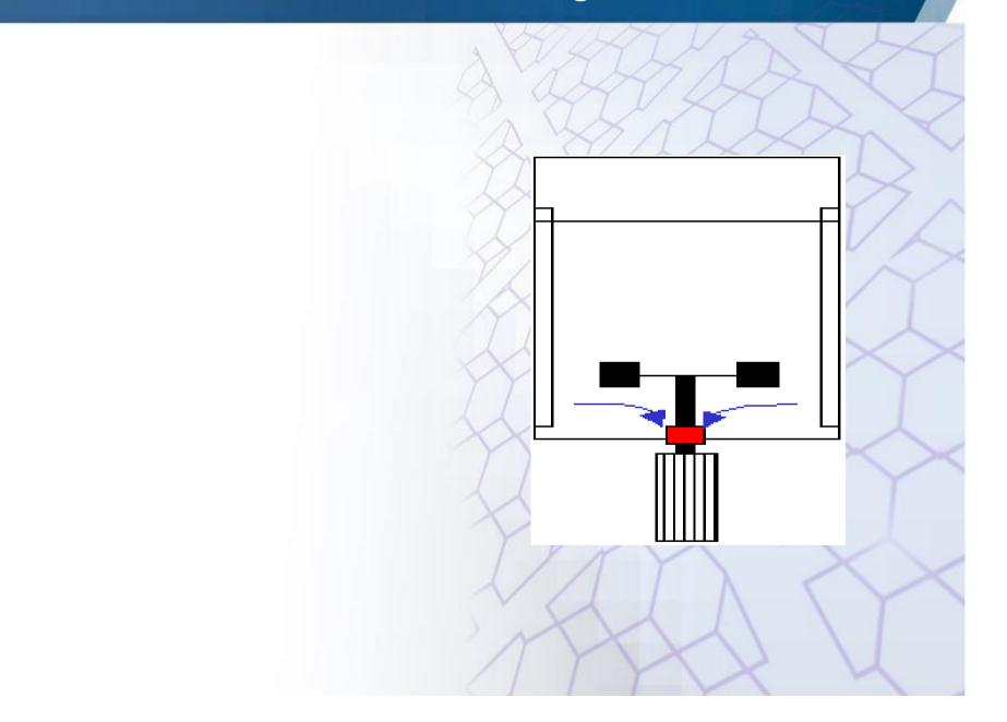
Bottom entry agitators tend to require more maintenance than top entry impellers due to the formation of crystals and other solids in the seals.
