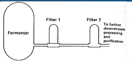
Figure representing the Filtration system for the removal of cells and cell debris form an animal cell culture fermentation.(Pall Process Filtration Ltd., Portsmouth, U.K.).
