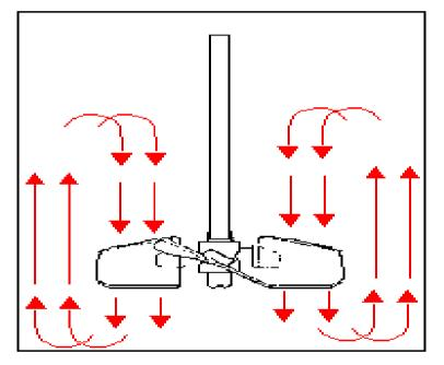
With axial impellers, the liquid is pushed in a downward direction; that is, along the axis of the reactor.
