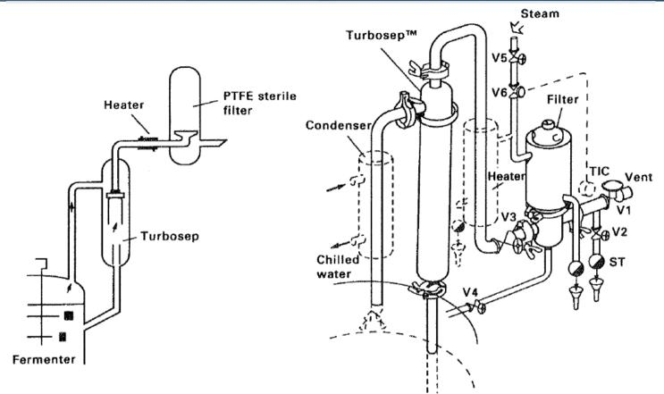
A mechanical separator and hydrophobic filter system for the sterilization of offgas from a fermenter. Left. Cut-away diagram. Right. Equipment arrangement, showing steam supply. VI-V6, valves; O, steam, traps
