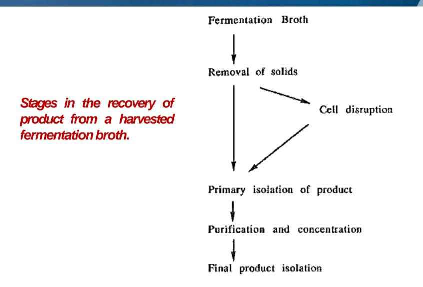
In the next stage, the broth is fractionated or extracted into major fractions using ultrafiltration, reverse osmosis, adsorption/ ion-exchange/gel filtration or affinity chromatography, liquidliquid extraction, two phase aqueous extraction or precipitation.
