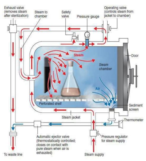
An autoclave. The entering steam forces the air out of the bottom (blue arrows). The automatic ejector valve remains open as long as an air-steam mixture is passing out of the waste line. When all the air has been ejected, the higher temperature of the pure steam closes the valve, and the pressure in the chamber increases.
