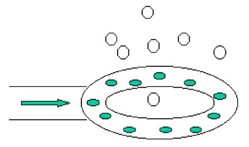
A sparger ring consists of a hollow tube in which small holes have been drilled. A sparger ring is easier to clean than porous materials and is less likely to block during a fermentation.
