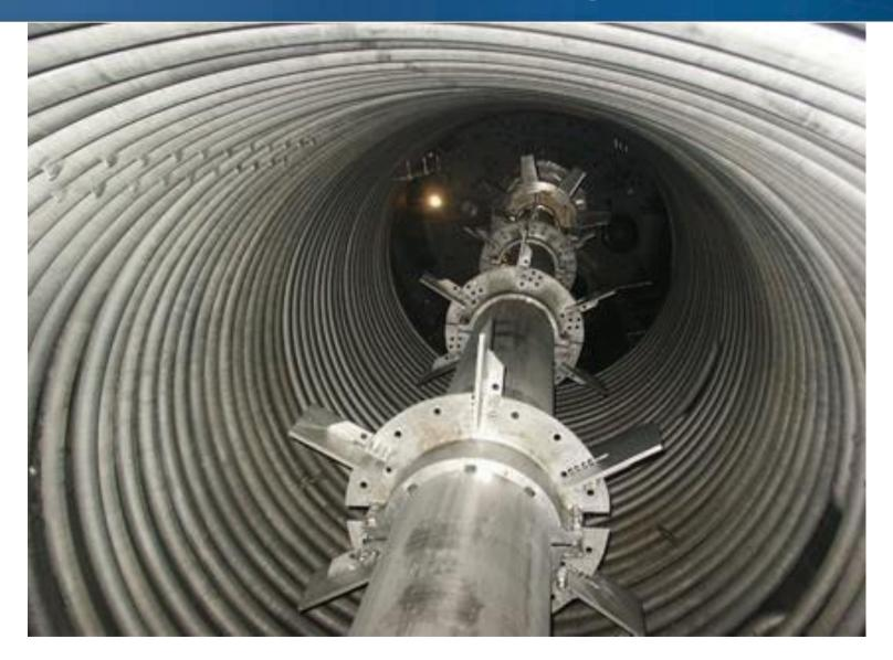
The impeller shaft can enter from the **bottom** of the tank or from the **top**. A top entry impeller ("overhung shaft") is more expensive to install as the motor and the shaft will need to be structurally supported:
