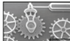
MicroElectroMechanical (MEMS) devices 10-100 \mu\text{m} wide
