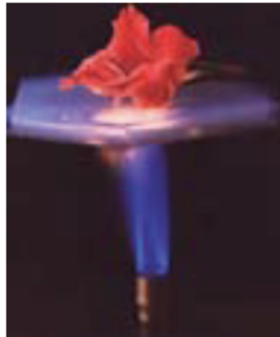
The thermal insulating properties of a silica aerogel
