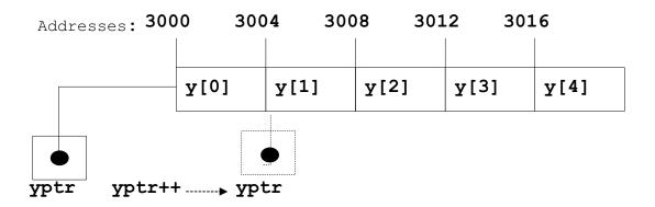
This diagram shows how an array occupies space in the memory. Suppose, we have an integer array named y and yptr is a pointer to an integer and is assigned the address of the first element of the array. As this is an integer array, so the difference between each element of the array is of four bytes. When the yptr is incremented, it starts pointing to the next element in the array.
