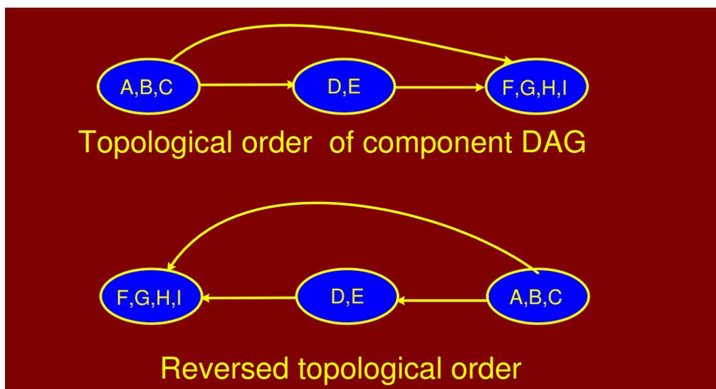
Figure 8.37: Reversed topological sort of component DAG
