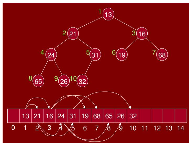
Figure 4.1: A min-heap
