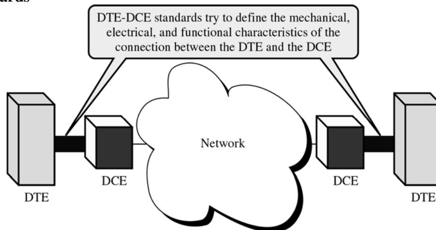
Many standards have been developed to define the connection b/w the DTE and a DCE
