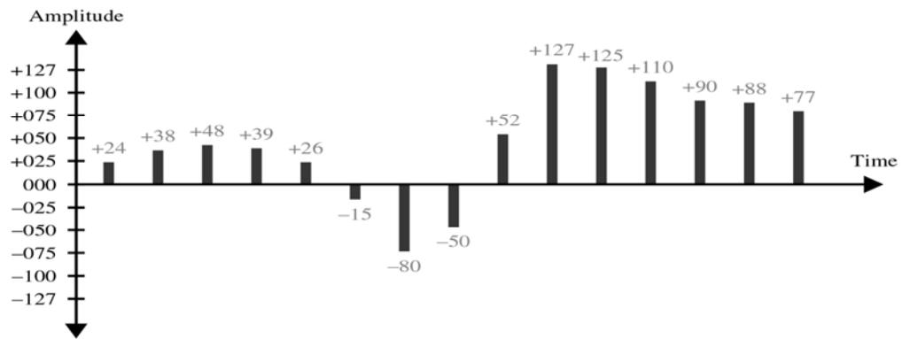
Figure shows a simple method of assigning sign and magnitude values to quantized samples
