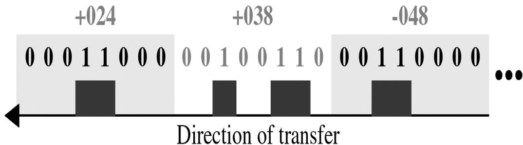
Figure shows the result of PCM of original signal encoded finally into a unipolar signal
