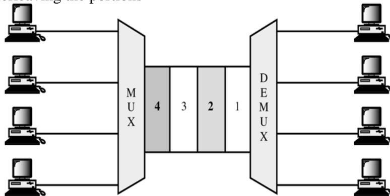
In fig, same link is used as in FDM. However, here the link is shown sectioned by time rather than frequency In TDM fig, portions of signals 1, 2, 3 and 4 occupy the link sequentially
