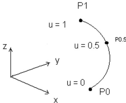
**Figure 2:** A plane curve defined by three points
