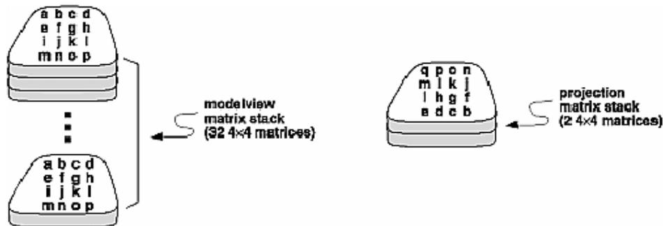
**Figure 20** : Modelview and Projection Matrix Stacks
