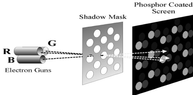
A **shadow-mask** is used which has holes aligned with the dots so that each gun can fire beam to corresponding dot only.
