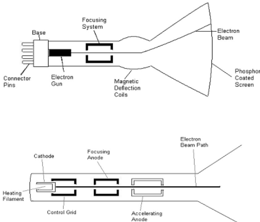
**Intensity of the electron beam is controlled** by setting voltage levels on the control grid, a metal cylinder that fits over the cathode. A high negative voltage applied to the control grid will shut off the beam by repelling electrons and stopping them from passing through the small hole at the end of the control grid structure. A smaller negative voltage on the control grid simply decreases the number of electrons striking the phosphor coating on the screen.
