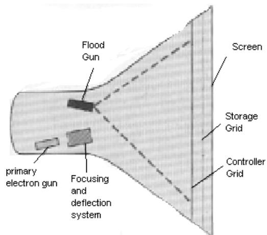
**Primary gun** is used to store the picture pattern whereas **flood gun** maintains the picture display.
