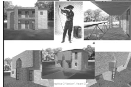
Another interesting simulation is **interactive walk through**. A sensing system in the headset keeps track of the viewer's position, so that the front and back of objects can be seen as the viewer walks and interacts with the displays. Similarly given below is a figure using a headset and a **data glove** worn on the right hand?
