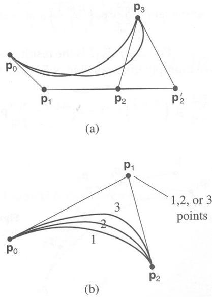
Figure 5: Modifying the shape of a Bezier curve.
