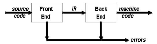
The figure above shows the structure of a two-pass compiler. The front end maps legal source code into an intermediate representation (IR). The back end maps IR into target machine code. An immediate advantage of this scheme is that it admits multiple front ends and multiple passes.
