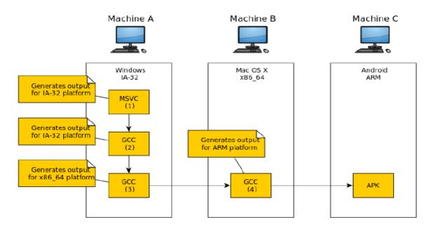
Picture of cross compile like GCC for compilation of C code and generating code for multiple platforms.
