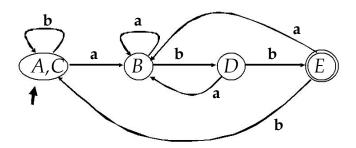
We can construct an optimized acceptor with the following structure:
