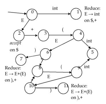
In order to remember the state the DFA goes into on a symbol, the parser stores the DFA state in the stack along with the symbol. Initial entry in the stack will be '<dummy,0>'.
