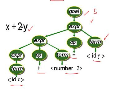
The parse tree captures all rewrite during the derivation. The derivation can be extracted by starting at the root of the tree and working towards the leaf nodes.
