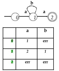
The rows correspond to states. The characters of the alphabet set appear in columns. The cells of the table contain the next state. This encoding makes the implementation of the FA simple and efficient. It is equally simple to simulate or run the FA given an alphabet and a string of the language and its associated alphabet set  $\sum$ . The C++ code shows such a FA simulator.
