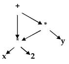
If the value of  $\mathbf{x}$  does not change between uses of  $\mathbf{x}^*\mathbf{2}$ , the compiler can generate code that evaluates the subtree once and uses the result twice.
