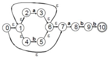
The start state of equivalent DFA is  $\varepsilon$  -*closure(0)*, which is  $A = \{0,1,2,4,7\}$ ; these are exactly the states reachable from state 0 via  $\varepsilon$  -transition. The algorithm tells us to mark A and then compute  $\varepsilon$  -*closure(move(A,a))*
