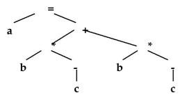
ASTs have been used in many practical compiler systems such as sourceto-source systems, automatic parallelization tools, pretty-printing etc.
