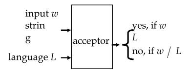
The acceptor is based on Finite Automata (FA). A Finite Automaton consists of
