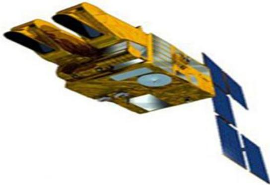
Spot satellite is a commercial high resolution optical imaging earth observation satellite system operating from space. It is run by spot image. Spot 1 was launch in December 31, 1990 and spot 5 in May 4, 2002 with 2.5 meter resolution. However spot 7 launched in 2014.
