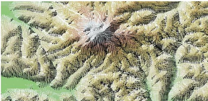
**Hachure** is method of representing the relief by means of sets of finely-drawn disconnected lines which indicate the direction of water flow. It does not show the absolute height. They are a form of shading, although different from the one used in shaded maps. Hachures are
