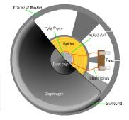
with a substance to improve its performance) are still in use today and can provide good quality sound. Plastics (e.g. Polypropylene), metals (e.g. aluminum), and composite materials (e.g. fiber-reinforced materials) are also used as diaphragm materials.
