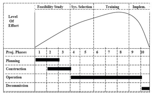
Figure 5.10: Project Life Cycle: Nuclear Power Station Project
