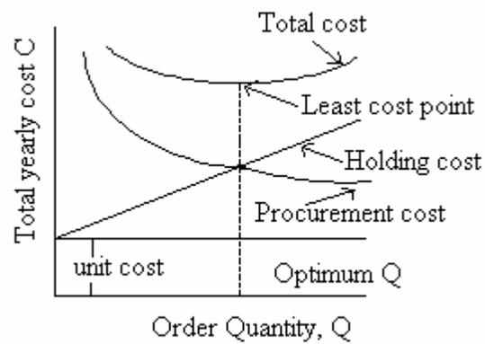
In this model, at time  $t = 0$ , we order a quantity  $Q$  which is stored as maximum inventory,  $I_m$ . The time ' $t$ ' denotes the time of one period or it is the time between orders or it is the cycle time. During this time, the items are depleting and reaching a zero value at the end of time  $t$ . At time  $t$  another order of the same quantity is to be placed to bring the stock upto  $Q$  again and the cycle is repeated. Hence this is a fixed order quantity model.
